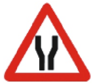
ROAD WIDENS AHEAD
