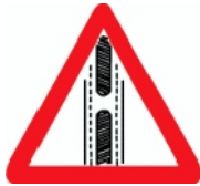
GAP IN MEDIAN
